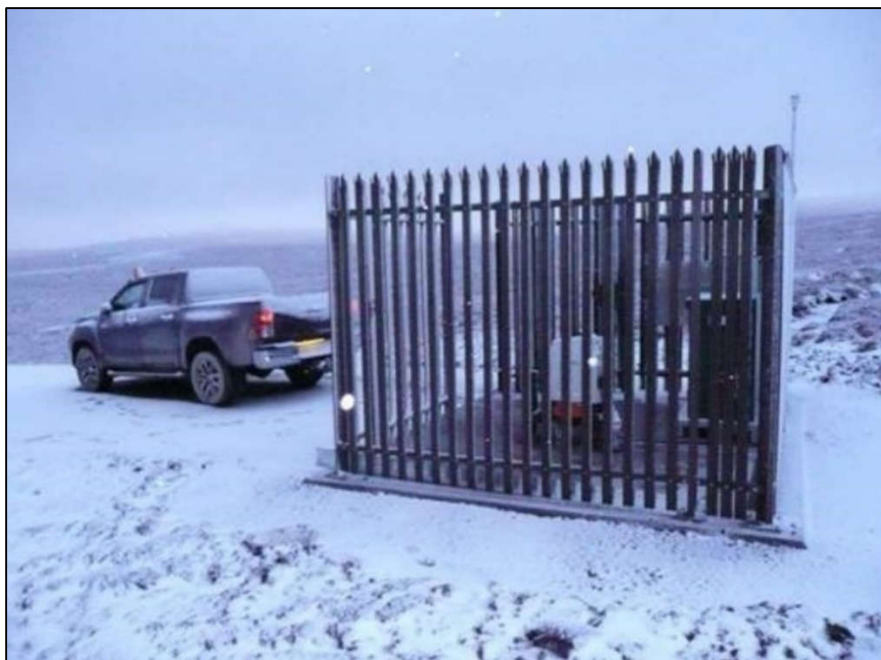
Figure 4-34: Photograph of a meteorological lidar facility on a wind farm with palisade fencing
